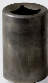
Forging of the blank socket with square drive and socket profile
