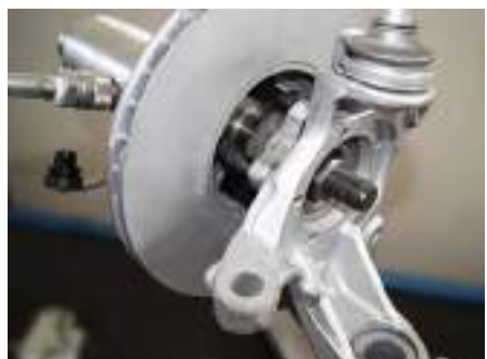
Dismantling of the wheel hub with the brake disc - change of wheel bearing
