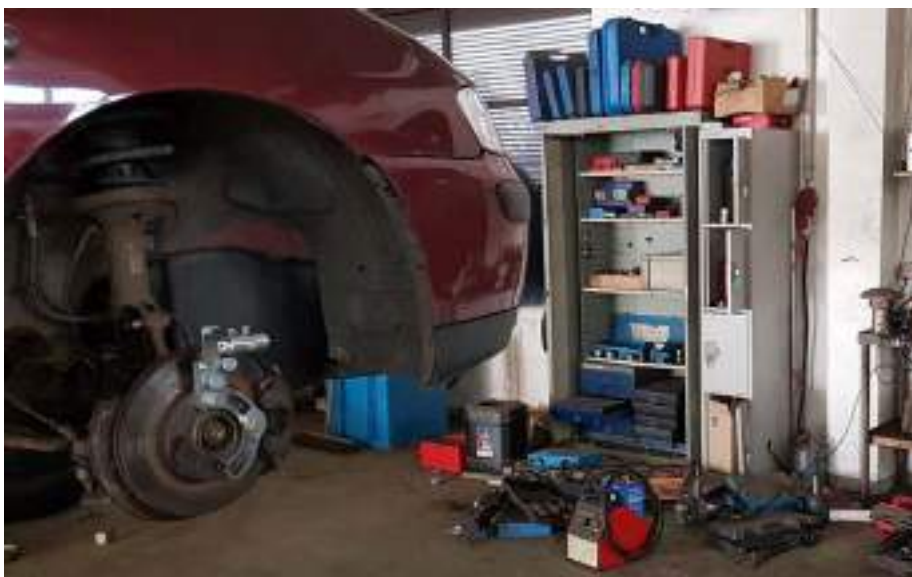
Replacing the suspension joints - Fixing the inclination value
