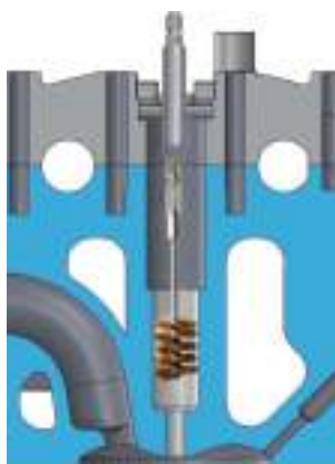
4 Special cleaning brushes for injector seat
