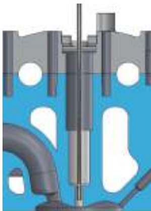
2 Sealing plugs for the injector housing
