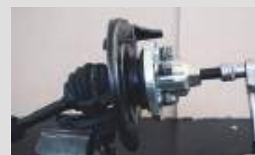
Pushing out the drive shaft, mechanically on the workbench
