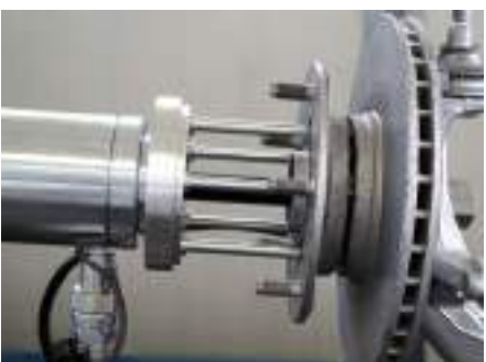
Detach the brake disc on the vehicle - change the brake disc
