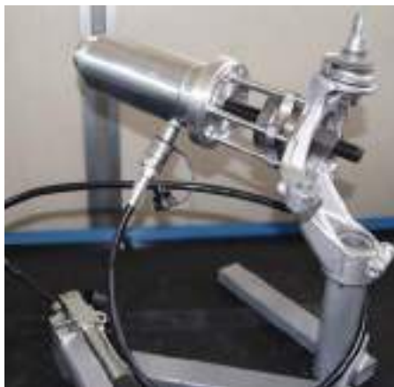
Dismatling of the wheel bearing on the vehicle - changing of the wheel bearing
