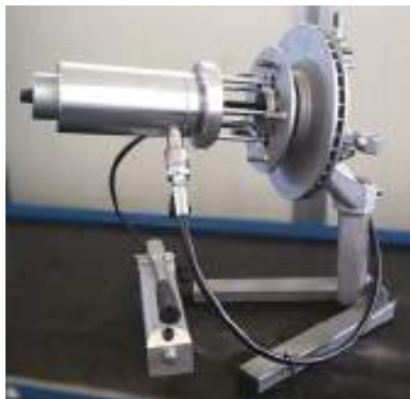
Dismantling of the wheel bearing - brake disc - wheel hubs - change the brake disc.
