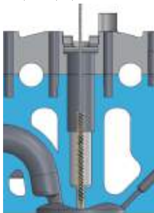
1 Pipe cleaners for cleaning the headquarters of injector sprayer
