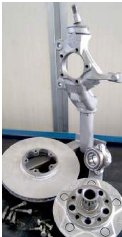
Dismatling of the wheel bearing on the vehicle - changing of the wheel bearing
