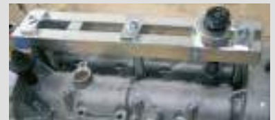
Extraction with 12TON mecadraulic cylinder
