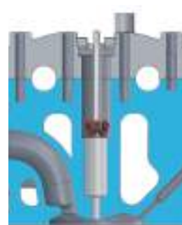
4 Finishing tool with cleaning brush
