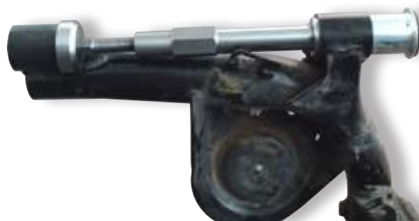
Removing silentblocks of Panda (4x4, cross, natural gas)
