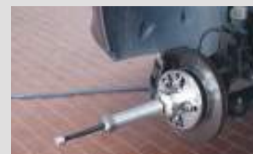
Pushing out the drive shaft, using a 16-Ton mechatronic screw, optional code GO1016
