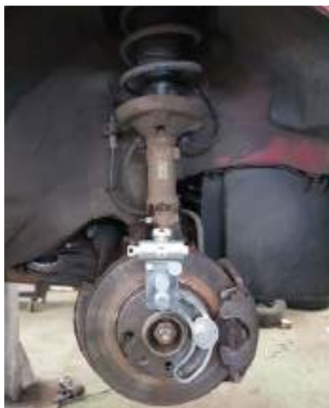
Replacing the tie-rod head - Fixing the toe-in value
